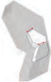
Refine wall fragment shape, ensure the fragment width change is not extreme
