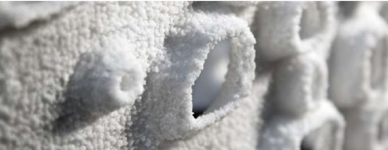
Close-up view of salt accretion in scaled prototype, GEOtube Tower
