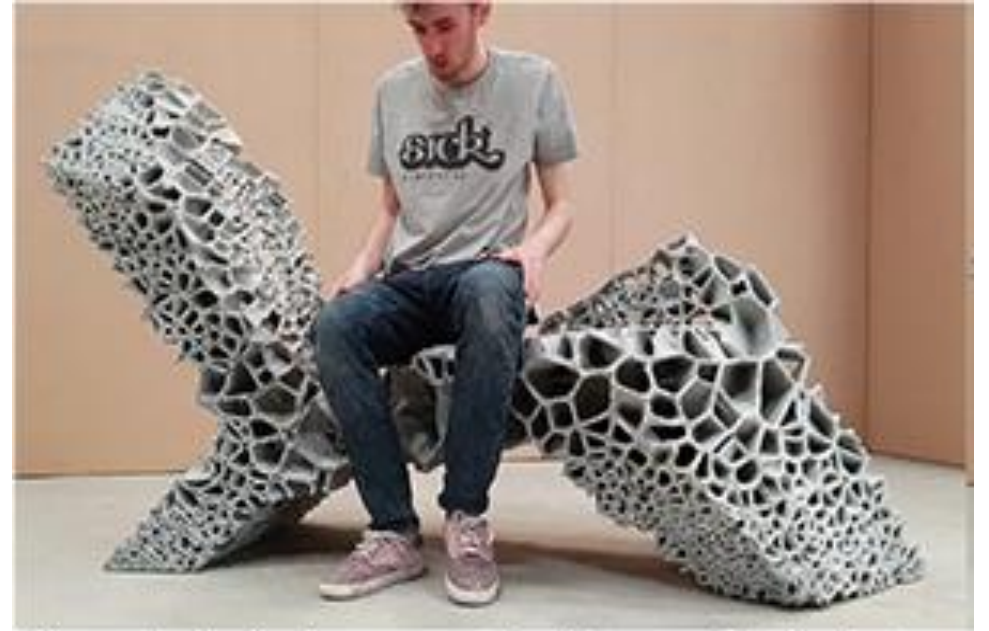
Figure 1: chaise longue made of thermoplastic elastomers (TPE) fabricated via robotic additive manufacturing: Variable Stiffness Chair, TU Delft
