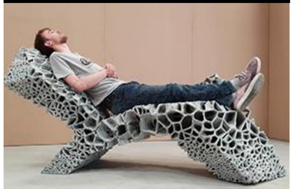
ers (TPE) fabricated via robotic additive manufacturing: Variable Stiffness Chair, TU Delft
