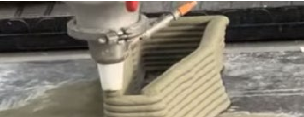
Close-up view of concrete additive 3d-printing, Vertico
