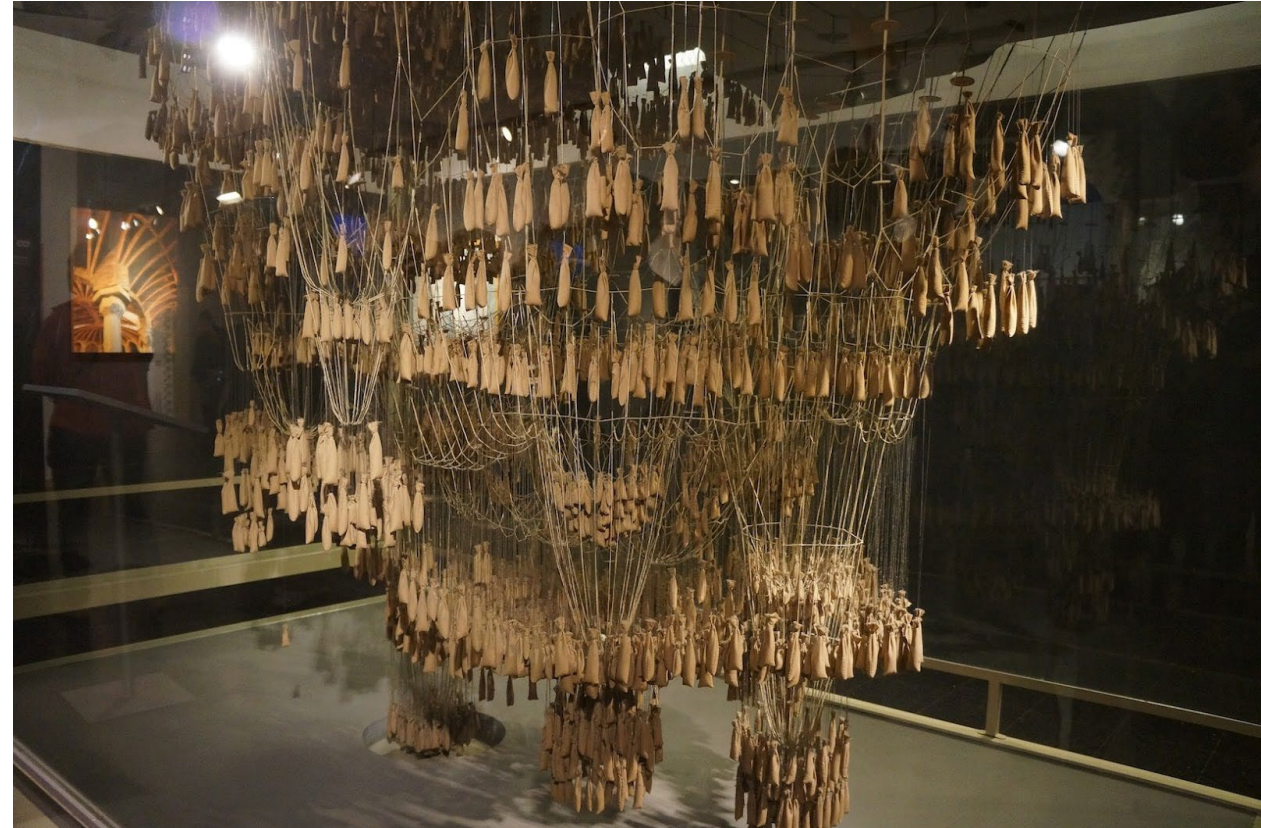
Nested Catenary Structure: Gaudi's Chain Model for Colonia Guell Chapel
