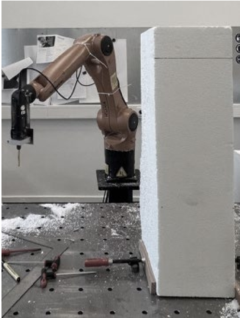
Subtractive method on foam using drill & robotic hand
