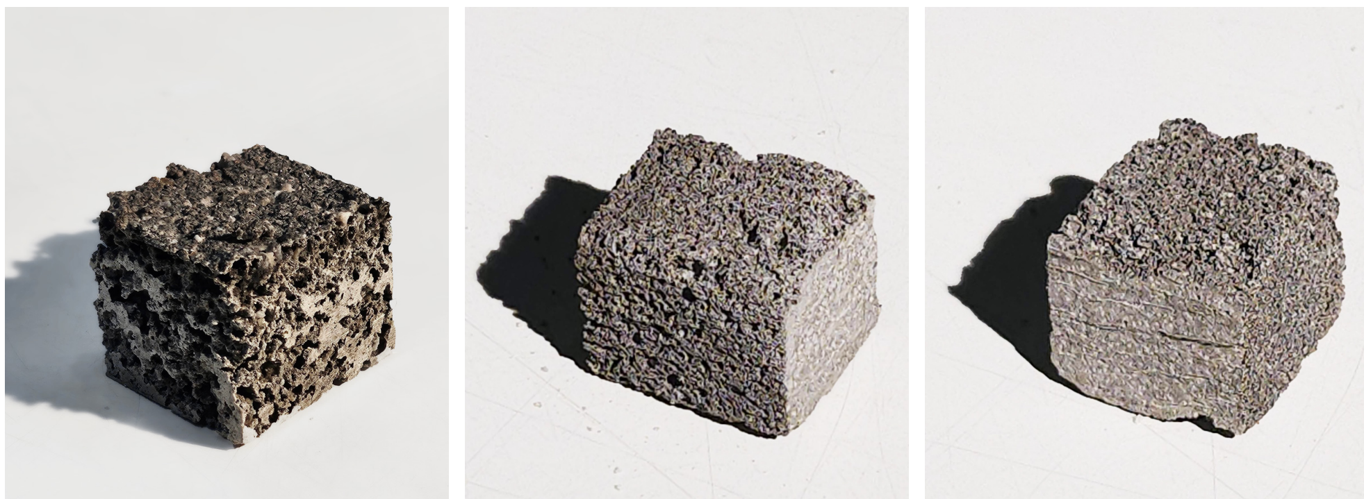
Fig3_Material specimens with varying particle size and porosity
