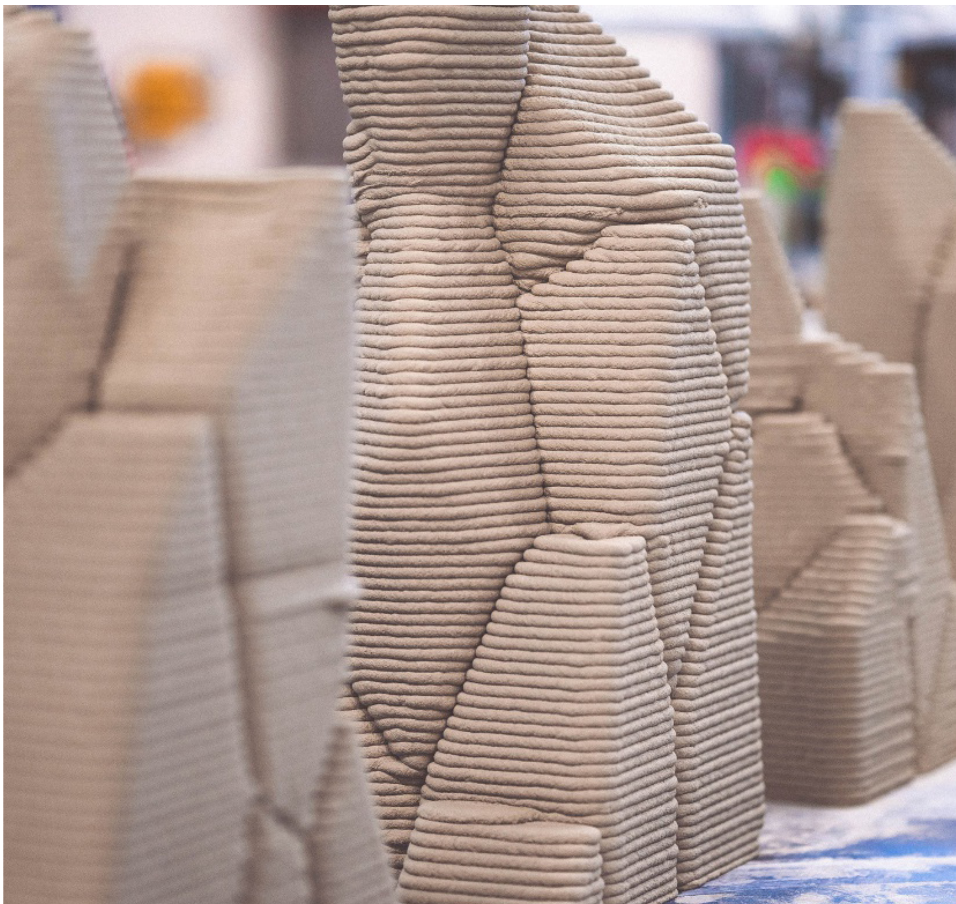
Fig1_Robotic 3D printed Rhizome 1.0 prototypes using concrete
